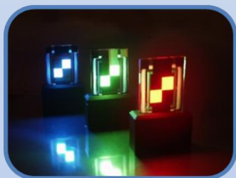
Some devices that use conductive glass: OLEDs (left) and DSCs (right).
